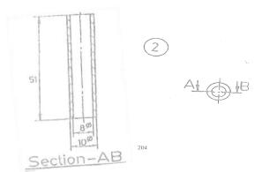
**Screw rod:** It has two parts A) Solid portion B) Threaded portion
