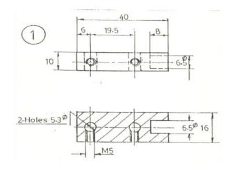
The total length of the plate is 40mm. The plate also has two holes in it. The diameter of both holes is similar to the diameter of plate No 4 i.e. 5.3mm.
